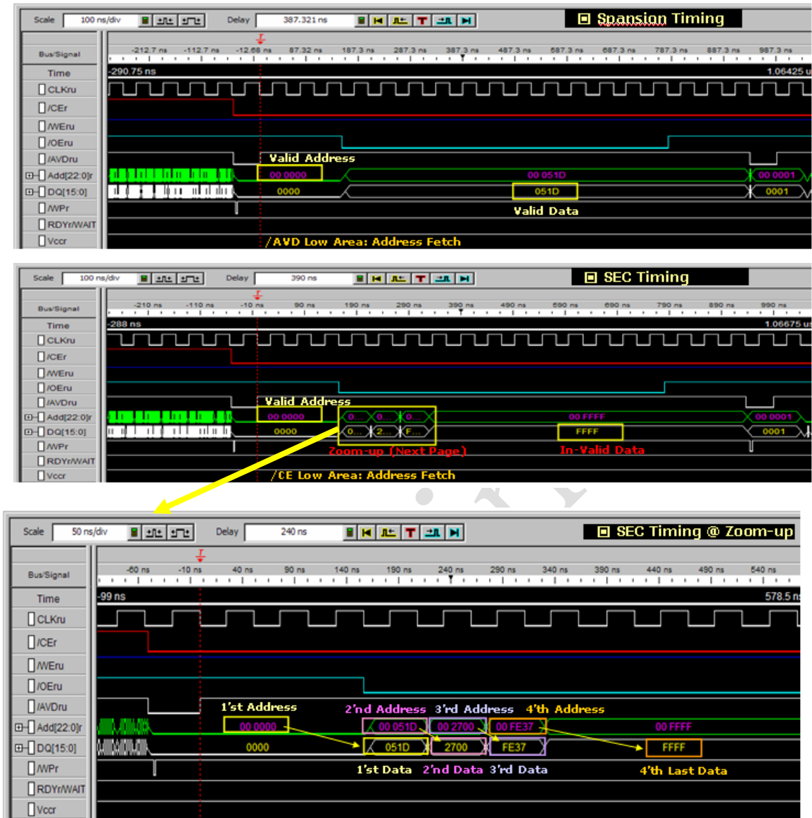
Figure 6 Timing of Address Fetch between SEC and Spansion
