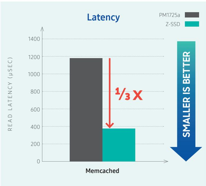
To summarize, these three test examples demonstrate Z-NAND SSD’s high degree of effectiveness in increasing throughput and lowering latency, across diverse domains. They show that the exceptional device-level performance of Z-NAND carries through to the application level, delivering an overall user-level performance increase and simplifying integration of the storage device in virtually any application.
