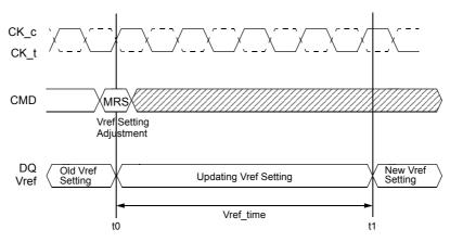
Figure 23. Vref\_time timing diagram
