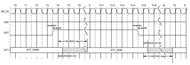
Figure 178. Asynchronous ODT Timing on DDR4 SDRAM with DLL-off
