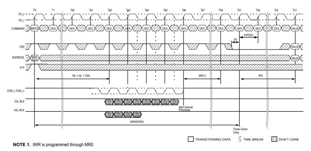
Figure 145. Power-Down Entry After Write with Auto Precharge
