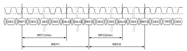
Figure 11. On-the-fly Refresh Command Timing
