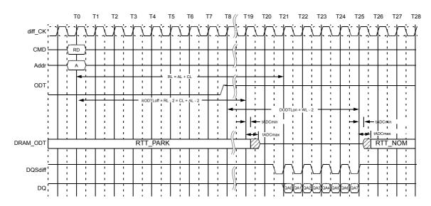
Figure 175. Example: CL=11, PL=0; AL=CL-1=10; RL=AL+PL+CL=21; CWL=9; DODTLon=AL+CWL-2=17; DODTLoff=AL+CWL-2=17;1tCK preamble)
