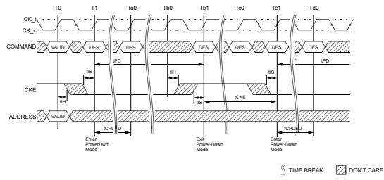
Figure 152. Power-Down Entry/Exit Clarification
