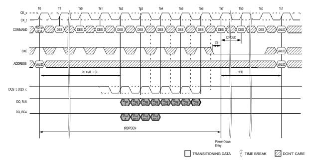
Figure 144. Power-Down Entry after Read and Read with Auto Precharge
