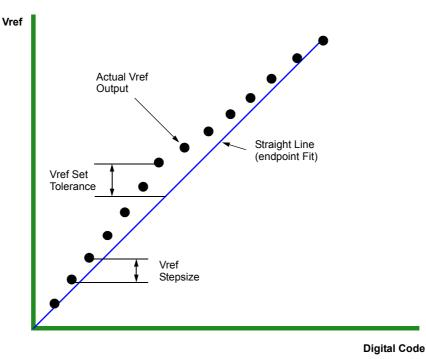
Figure 22. Example of Vref set tolerance(max case only shown) and stepsize
