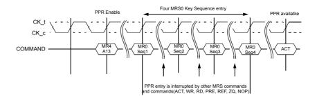
Figure 165. Timing Diagram for soft PPR Key Sequence
