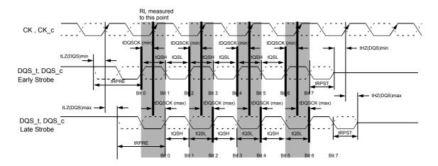
1. Within a burst, rising strobe edge can be varied within tDQSCKi while at the same voltage and temperature. However incorporate the device,
