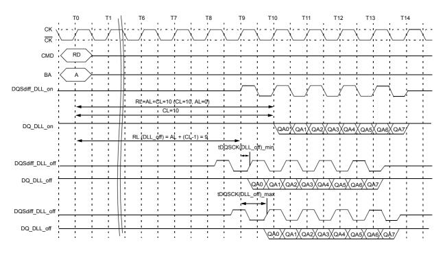
Figure 7. READ operation at DLL-off mode
