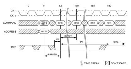
Figure 150. Precharge/Precharge all Command to Power-Down Entry
