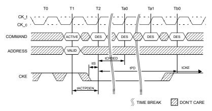
Figure 149. Activate Command to Power-Down Entry
