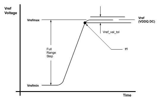
Figure 27. Vref full step from Vrefmin to Vrefmax case
