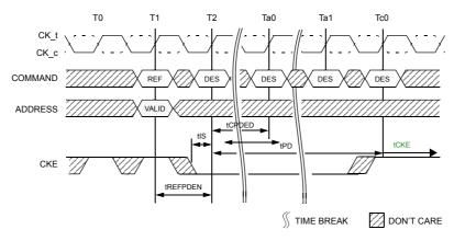
Figure 148. Refresh Command to Power-Down Entry
