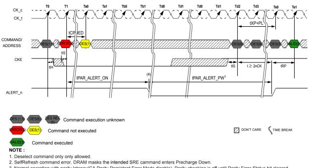
Figure 44. CA Parity Error Checking - PDE/PDX
