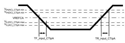
Figure 160. CS\_n and Input A Slew Rate Definition
