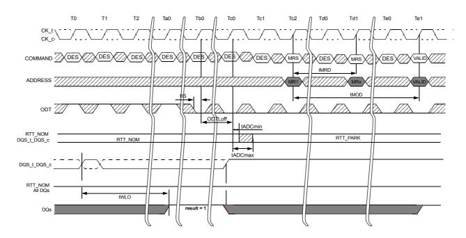
Figure 10. Timing details of Write leveling exit
