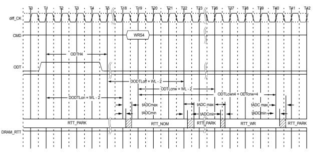
Figure 174. Synchronous ODT example with BL=4, CWL=9, AL=10, PL=0; DODTLon/off=WL-2=17, ODTcnw=WL-2=17
