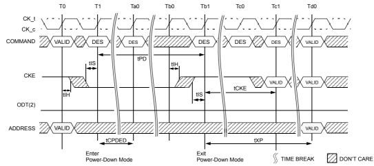
**NOTE :** 1. VALID command at T0 is ACT, DES or Precharge with still one bank remaining open after completion of the precharge command. 2. ODT pin driven to a valid state. MR5 bit A5=0 (default setting) is shown.
