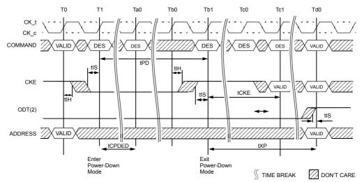
NOTE : 1. VALID command at T0 is ACT, DES or Precharge with still one bank remaining open after completion of the precharge command. 2. ODT pin driven to a valid state. MR5 bit A5=1 is shown.
