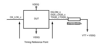
Figure 181. ODT Timing Reference Load
