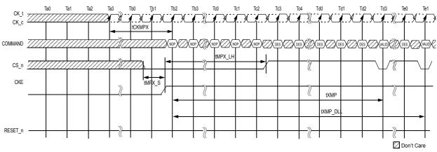
Figure 157. Maximum Power Saving Mode Exit Sequence
