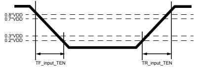
Figure 159. TEN Input Slew Rate Definition
