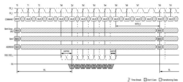
**NOTE :** 1. tWTR\_S : Delay from start of internal write transaction to internal read command to a different Bank Group.
