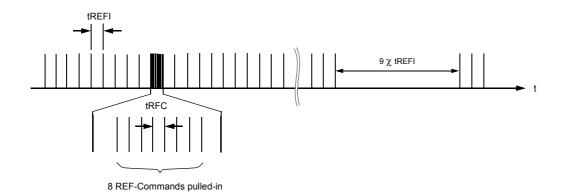
Figure 139. Pulling-in Refresh Commands (Example of 1X Refresh mode)
