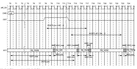
ODTLcnw = WL-2 (1tCK preamble), WL-3 (2tCK preamble) ODTLcwn = WL+2 (BC4), WL+4(BL8) w/o CRC or WL+5,5 (BC4, BL8 respectively) when CRC is enabled.
