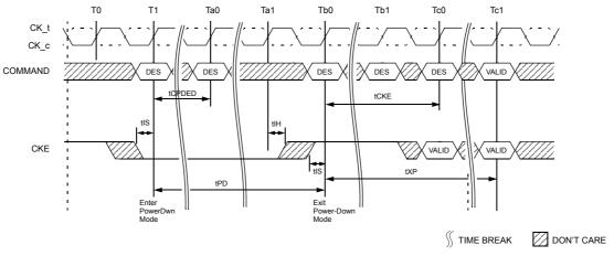
Figure 147. Precharge Power-Down Entry and Exit
