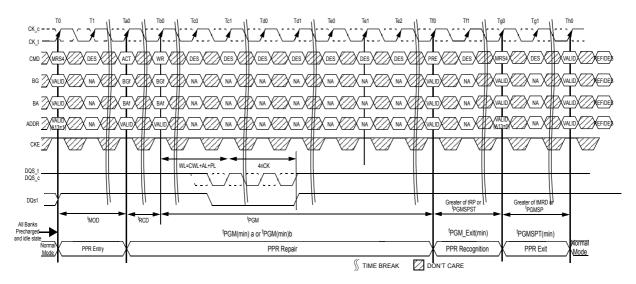
Figure 167. Fail Row Repair (WR Case)
