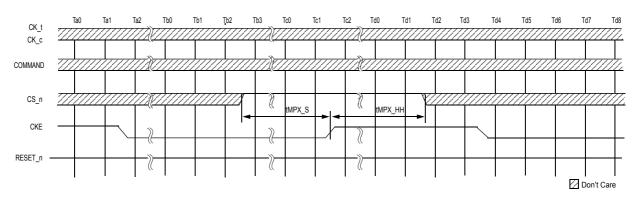
Figure 156. CKE Transition Limitation to hold Maximum Power Saving Mode
