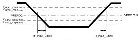
Figure 161. Input B Slew Rate Definition
