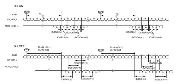
Figure 162. tDQSCK Definition Difference between DLL ON and DLL OFF
