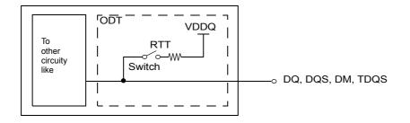
Figure 171. Functional Representation of ODT
