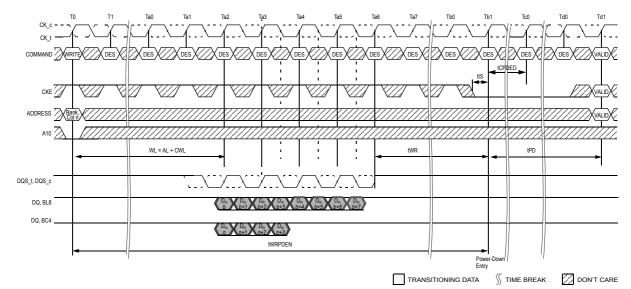
Figure 146. Power-Down Entry after Write
