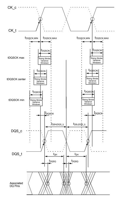
Figure 63. READ Timing Definition
