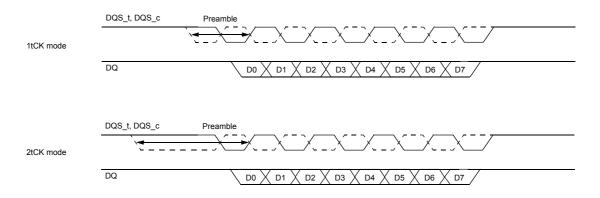
The timing diagrams contained in Figure 60, Figure 61 and Figure 62 illustrate 1 and 2 tCK preamble scenarios for consecutive write commands with tCCD timing of 4, 5 and 6 nCK, respectively. Setting tCCD to 5nCK is not allowed in 2 tCK preamble mode
