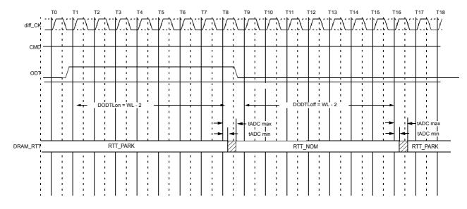
Figure 173. Synchronous ODT Timing Example for CWL=9, AL=0, PL=0; DODTLon=WL-2=7; DODTLoff=WL-2=7
