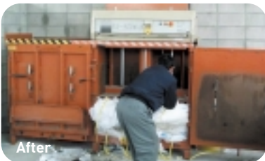
Waste vinyl is recycled and effectively managed using a recycling compressor.
