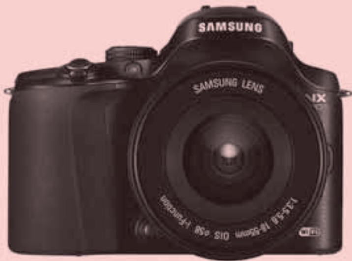
Compact System Camera, NX20 This mirrorless camera system has a 20.3 megapixel high-quality APS-C sensor that shoots 8 continuous frames a second.
